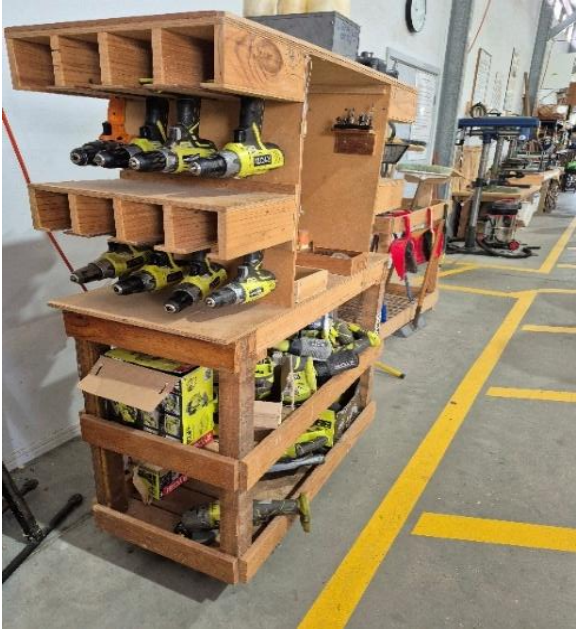
Power tool stand including charging station
